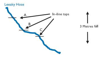
In the above example, in-line tap 'C' is inserted in the hose on the first metre of fall up the slope and the flow rate is adjusted at (for example) 2 litres (L) per metres (M) per hour where (M) equals the number of metres between 'C' and the end of the hose. Tap 'B' is adjusted for the flow rate required between B and C PLUS the flow rate from C downwards. Therefore tap 'A' would be set for the flow rates required from the start to 'A', plus the flow rates required through 'B' and 'C'.
