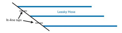
The in-line taps are placed in the feeder line at approximately each metre of fall and the flow rate adjusted to the appropriate water requirement for the number of metres of Leeaky Hose below each tap.
