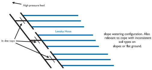
In the above diagram the single in-line tap feeding each three or more lines of Leeaky Hose is fed from a high-pressure line. The flow rates through each tap can be regulated for the individual soil type or plant needs.
