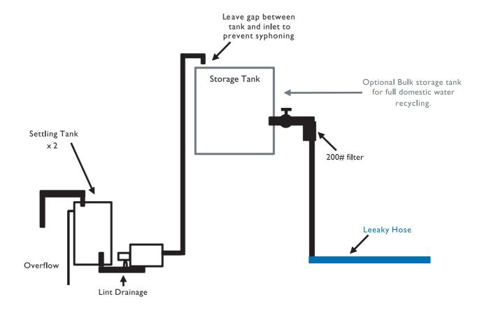
It pays to have two settling tanks (2 x 200 litre drums), so the washing machine hose can be alternated each day from tank to tank. Lint can be drained from the bottom of the settling tanks. Every now and then put some fresh water through the hose to flush out any soap residues.
